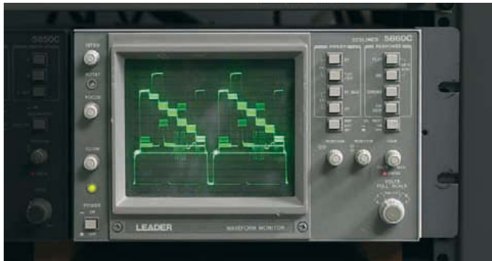
Figure 25-4. The waveform monitor measures every aspect of the television signal except color strength.
