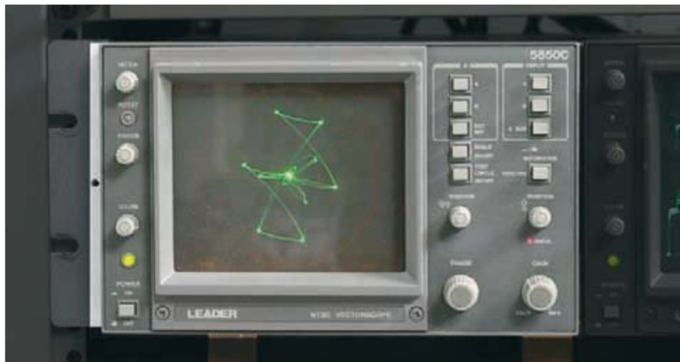
Figure 25-5. The vectorscope graphically measures a signal's color strength and adherence to industry standard settings.
