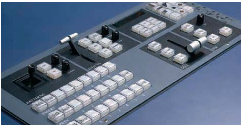
Figure 2-19. The production switcher allows the operator to send pictures from different cameras to the video recorder, simply by pushing a button or pulling a lever.
