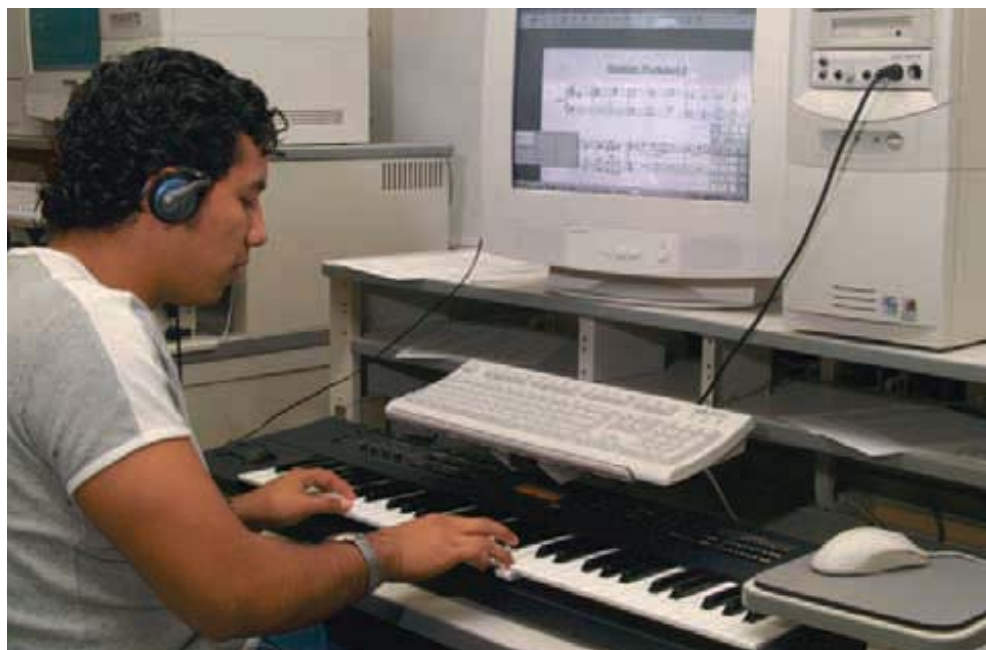
Figure 2-2. Using a Musical Instrument Digital Interface (MIDI) computer program, a composer sends notes directly from the keyboard to the computer. The notes are placed on sheet music and can be printed, so the music can be performed, recorded, and placed into the soundtrack of the production.
